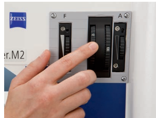
Ideal arrangement of the diaphragm slider and filter wheel in reflected-light
