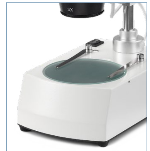
● Transparent stage plate for transmitted illumination
